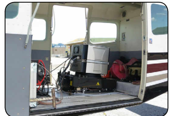
Below: UltraCam Eagle installed in the aircraft.
