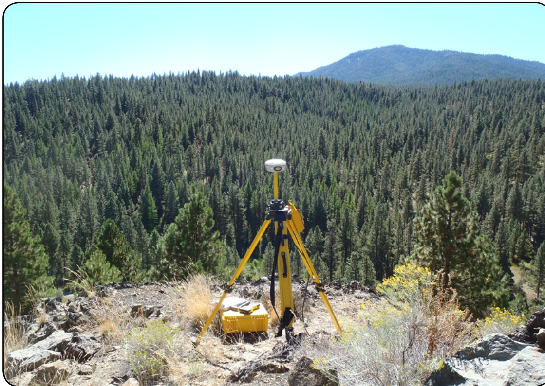
Trimble R8 (left) positioned over the GPS Monument Cap QB1364 (above).
