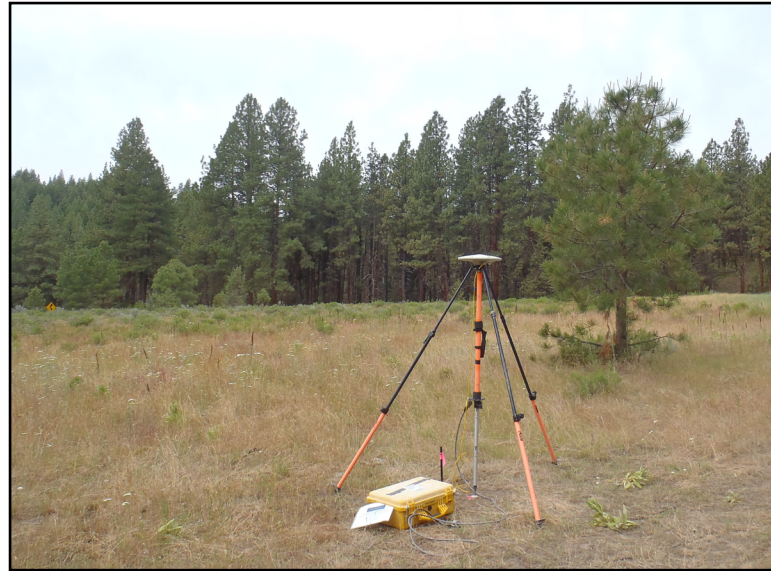
Left: Ground professional collecting Ground Check Points in the Crooked Ochoco study area
