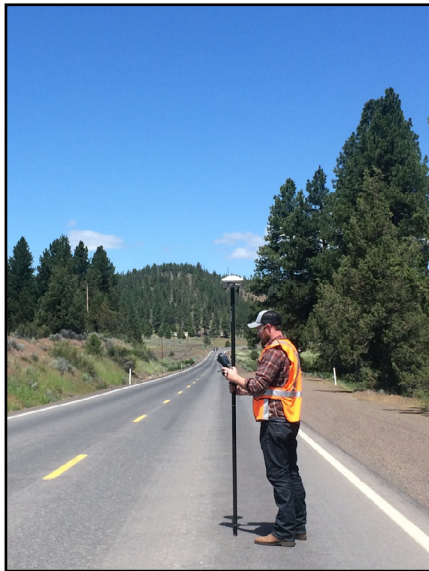
Left: Ground professional collecting Ground Check Points in the Crooked Ochoco study area
