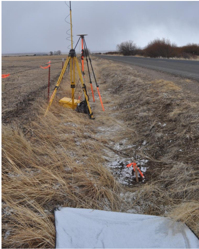
Figure 4. GPS base station set up with “space” blanket target set up near the control monument. The space blanket has a very low emissivity compared to the surrounding terrain and is detectable in the TIR imagery. The blankets were paired with small, catalytic heaters to quantify the accuracy of the TIR mosaic
