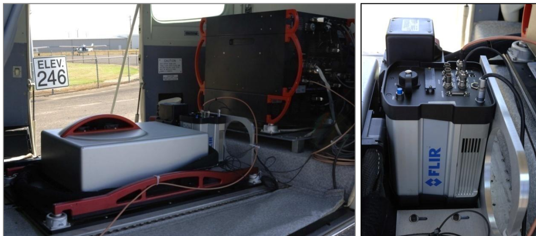
Figure 2 - WSI's FLIR SC6000 integrated with a Leica ALS50-Phase II LiDAR System installed in one of WSI's Cessana Caravans. The SC6000 utilizes the same GPS/IMU system as the LiDAR system for direct computation of image external orientation
