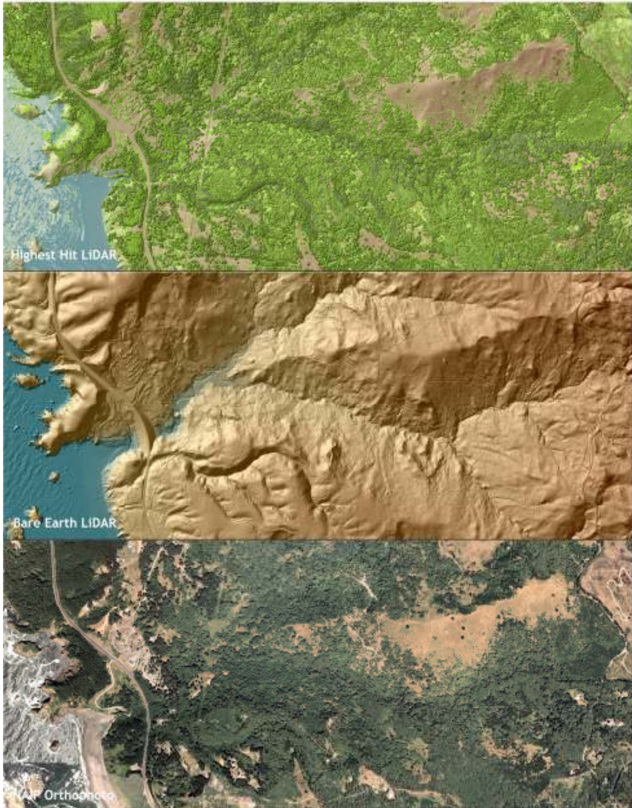
Figure 4.8. Whalehead and Coon Creek at terminus in ocean near Highway 101 (quad42124-b3). Top image derived from highest hit LiDAR, center image from bare earth LiDAR, lower image derived from NAIP orthophotos.
