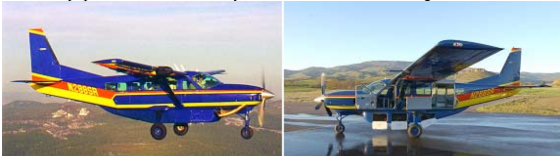
Figure 3. The Cessna Caravan 208 - A removable composite cargo pod provides housing for GPS equipment and the LiDAR system and other remote sensing sensors.
