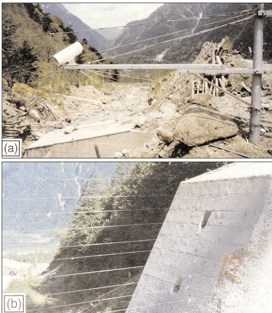
Figure 27. Examples of monitoring devices for debris flow warnings, (a)—a current gage and (b) a wire sensor system. (Photos from United Nations, 1996)
