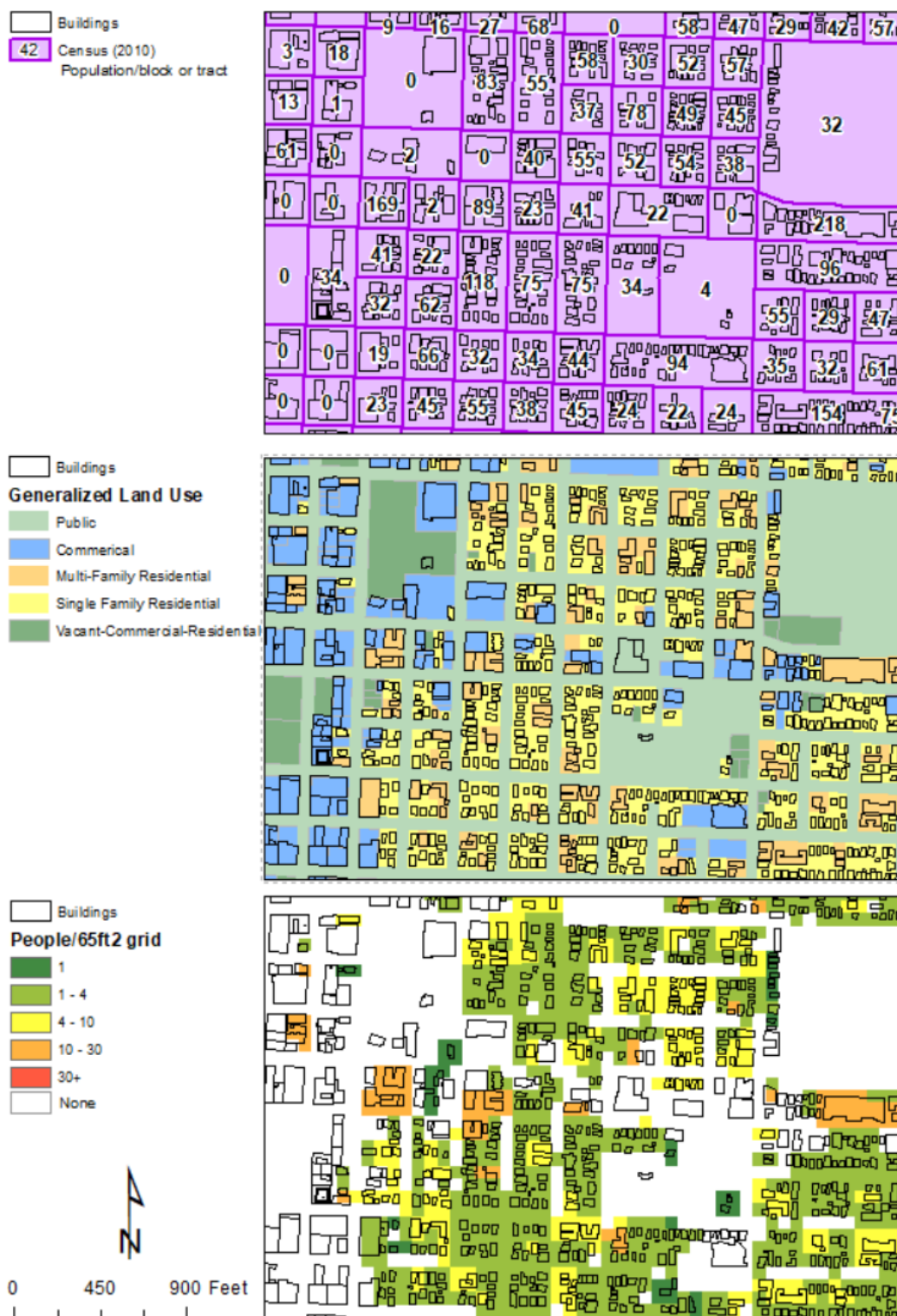
Figure 3-2. Dasymetric population distribution map input data and result examples.
