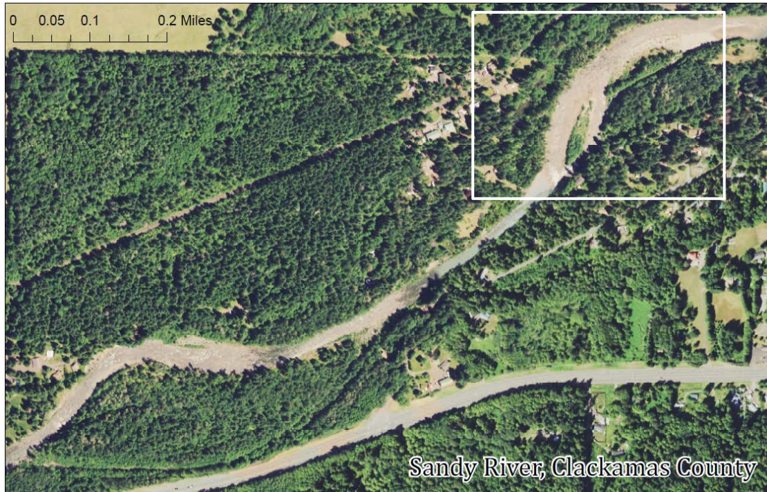
Figure 4-3. Example of a stream segment with aspects of both anastomosing and braided channel patterns. This segment was classified as anastomosing due to the presence of island bars with established vegetation present (upper-right, boxed area).
