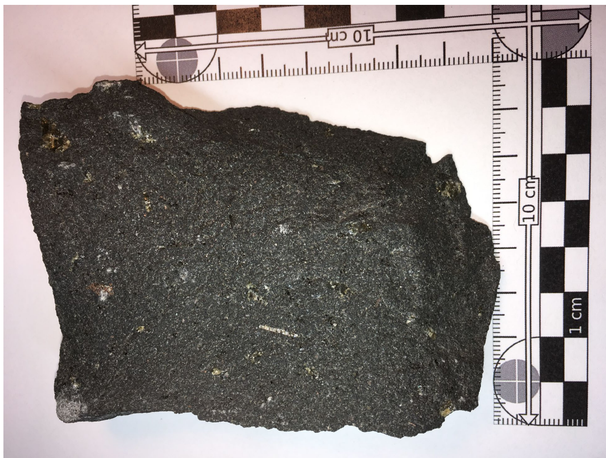
Figure 5-29. Hand sample of Basalt of Roza. Sample BJ18-25A.
