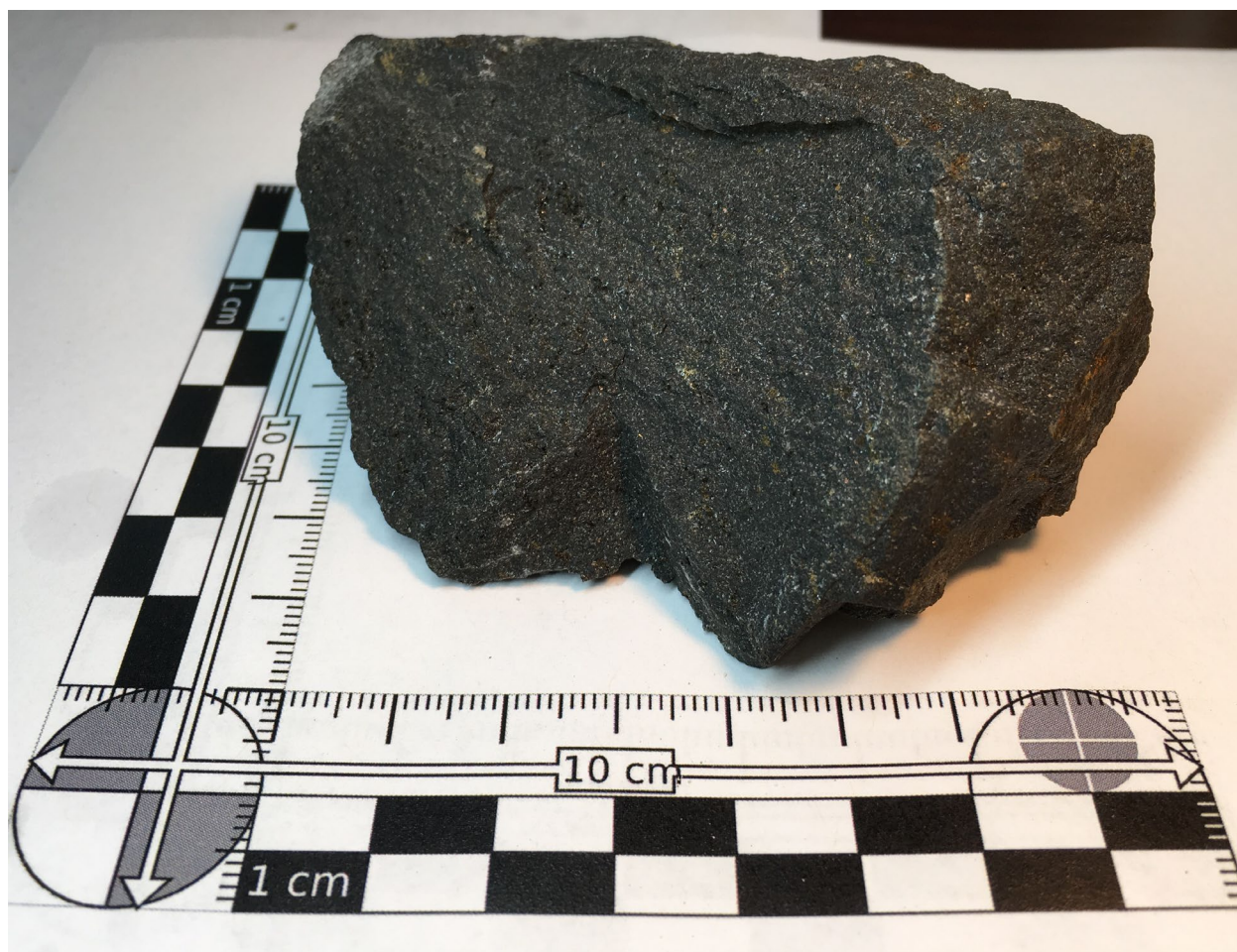
Figure 5-26. Hand sample of Basalt of Rosalia. Sample BJ18-199.
