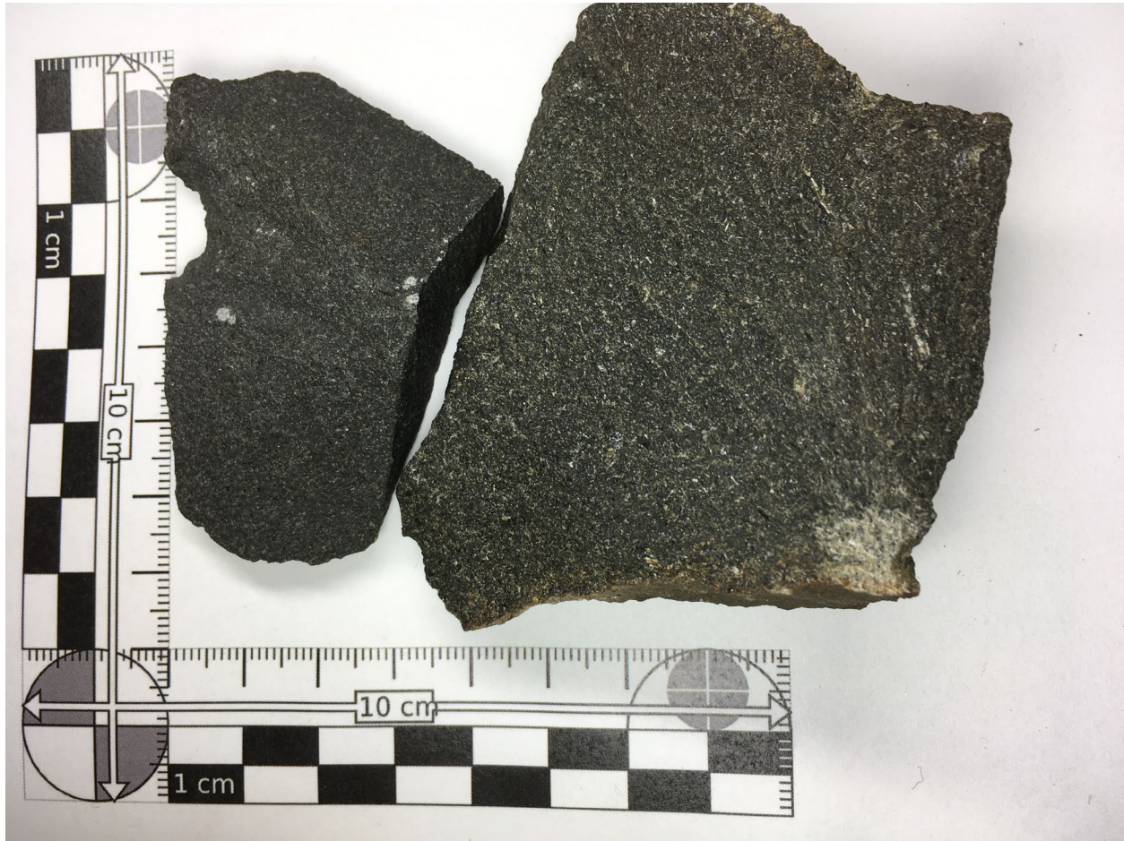
Figure 5-45. Hand samples of the Basalt of Sand Hollow. Smaller specimen is from the dense basal colonnade and is finer grained and has fewer plagioclase microphenocrysts than the majority of the flow, represented by the larger sample.
