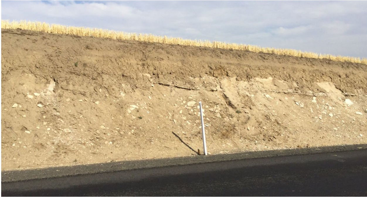
Figure 5-9. Cultivated loess (Qlc) exposed in a roadcut across a dune crest located at 679812 E, 5056227 N, view to east. Dipping resistant layers and angular float are caliche, cut height is ~ 4 m (13 ft).
