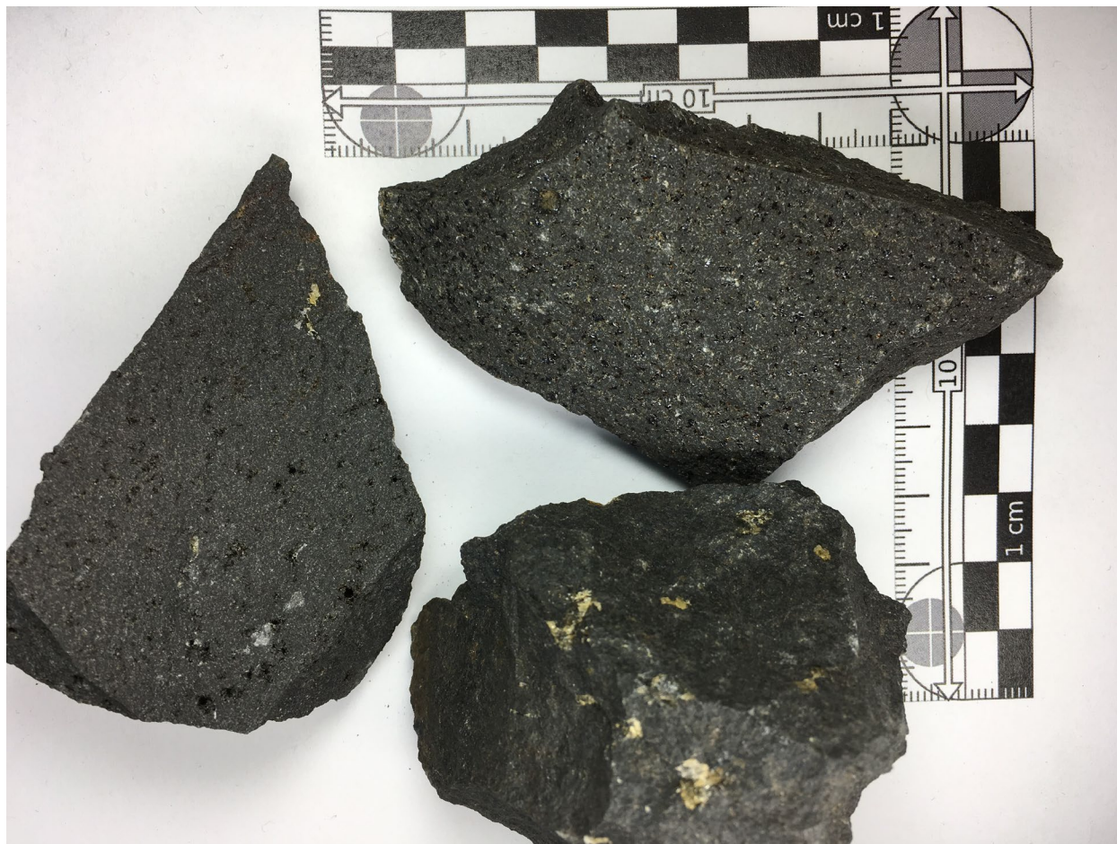
Figure 5-50. Hand samples of the Basalt of Ginkgo. Clear to yellow blocky plagioclase phenocrysts 2–10 mm in diameter occur with varying abundance.
