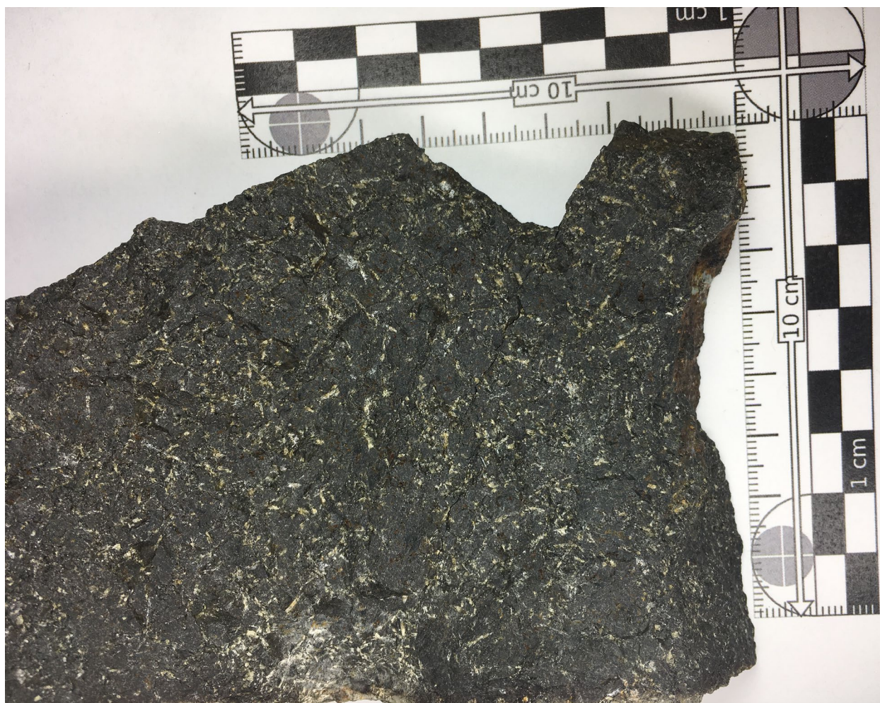
Figure 5-47 Hand specimen of “pegmatoid” Basalt of Sand Hollow Yellow and white flecks are lath-shaped plagioclase phenocrysts and microphenocrysts. Sample number BJ18-21, map code G11, location 677749 E, 5061963 N.
