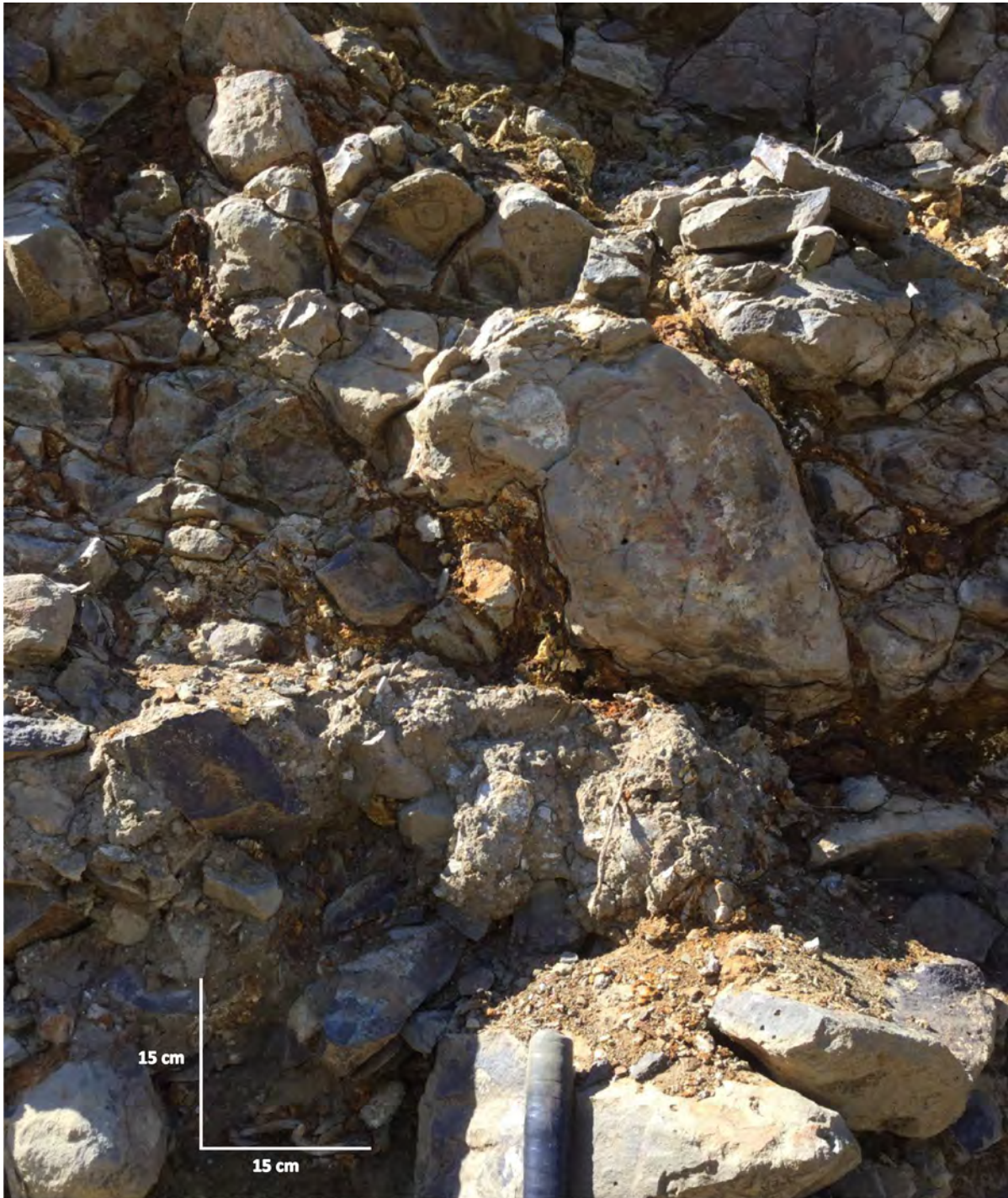
Figure 5-41. Hydrothermal alteration of the Basalt of Sand Hollow along U.S. Route 97 southeast of Biggs Junction. Red and yellow mixture of iron oxide and clays deposited along joints. Location 678472 E, 5061598 N, view to west.
