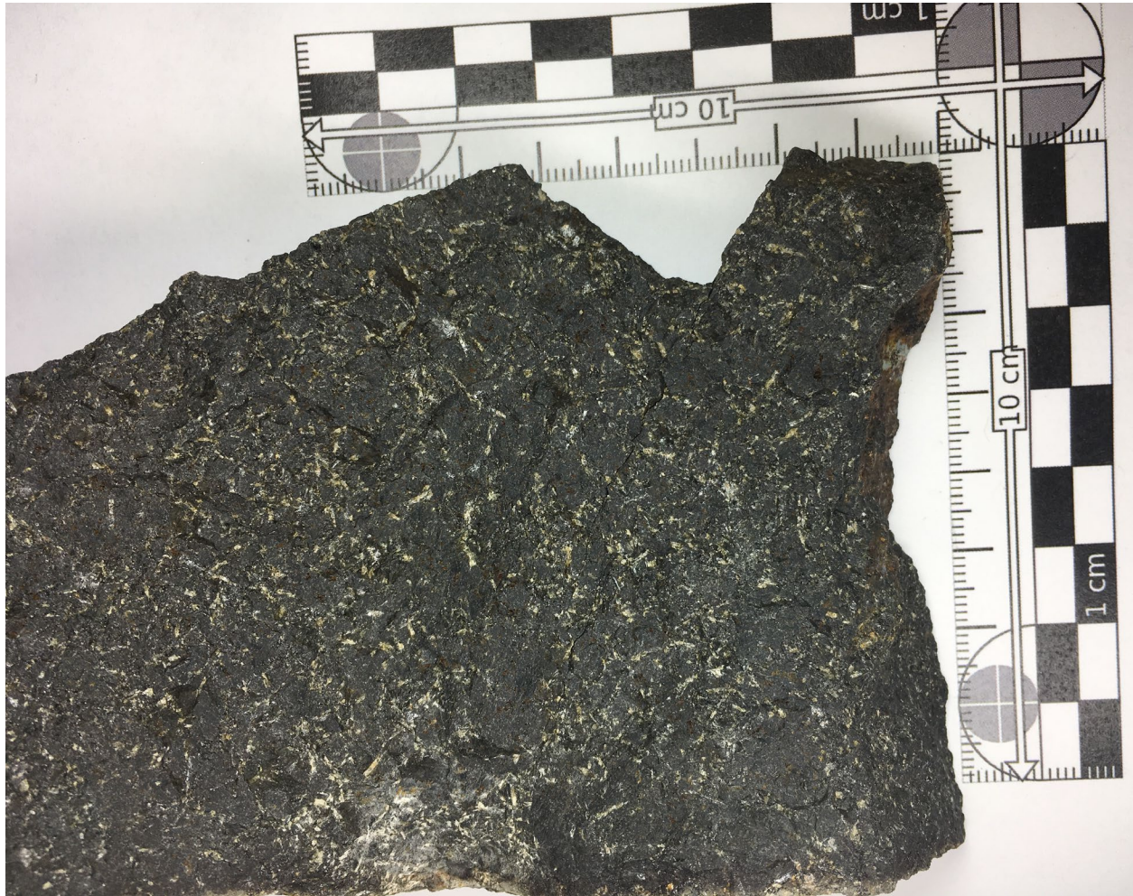
Figure 5-47 Hand specimen of “pegmatoid” Basalt of Sand Hollow Yellow and white flecks are lath-shaped plagioclase phenocrysts and microphenocrysts. Sample number BJ18-21, map code G11, location 677749 E, 5061963 N.
