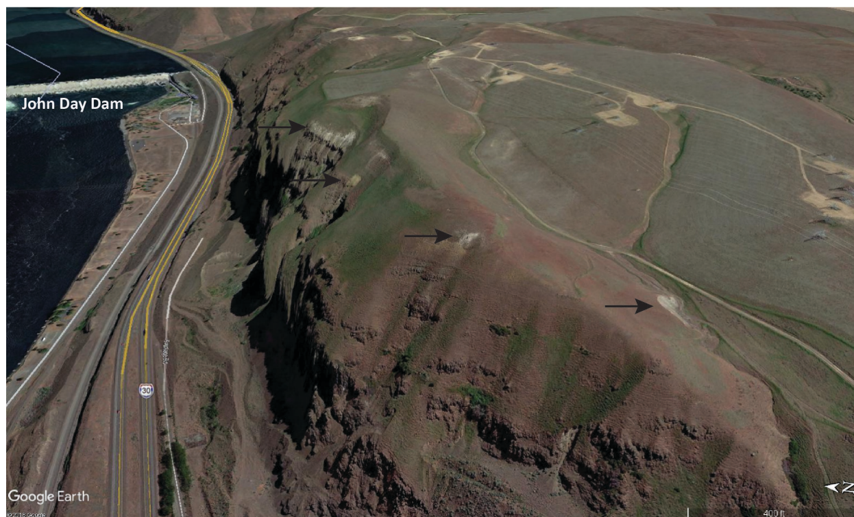
Figure 5-10. Google Earth™ view of the cliffs east of Rufus. Areas of white and yellow-tan sediment exposed above basalt (indicated by black arrows) are inferred to be bedded volcanoclastic sedimentary rocks of the Dalles Formation ( Tmdl ).
