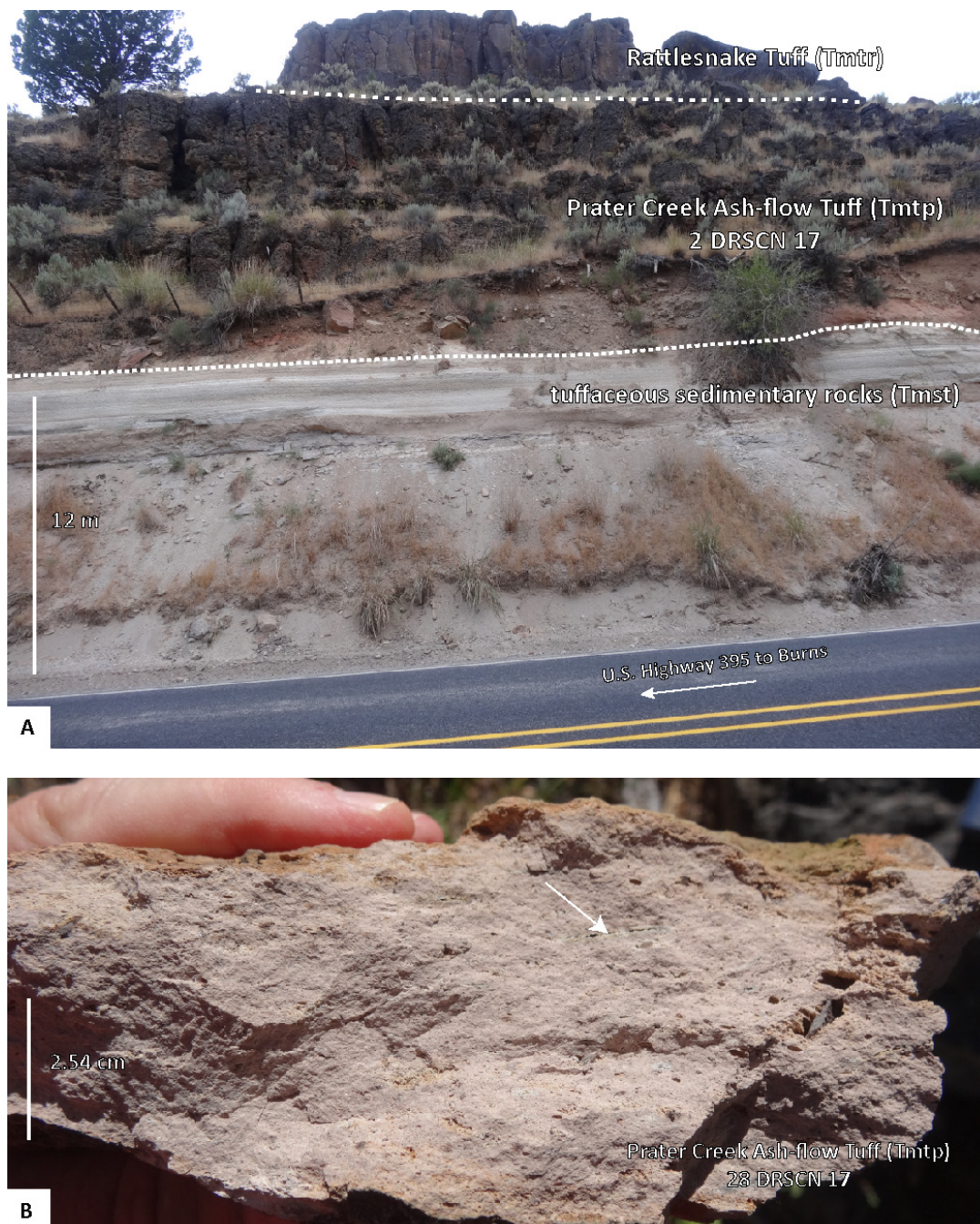
Figure 5-3. Field photograph of the Prater Creek Ash-flow Tuff (Tmtp). (A) The Prater Ash-flow Tuff, 7 to 8 mi (11 to 12 km) north of Burns, along the west side of U.S. Highway 395. The upper ledge, at skyline, is the welded part of the Rattlesnake Tuff (Tmtr). Tuffaceous sedimentary rocks (unit Tmst) underlie the Prater Creek Ash-flow Tuff (Tmtp). Photograph taken from U.S. Highway 395 looking west. (43.676596, -118.999331 WGS84 geographic coordinates; 4837896mE, 338836mN WGS84 UTM Zone 11 coordinates). Scale bar is 12 m (39.4 ft) high. (B) In hand sample, the devitrified welded groundmass contains fiamme (arrow), lithic fragments, and rare alkali feldspar crystals (43.741265, -118.914546 WGS84 geographic coordinates; 4844918mE, 345836mN WGS84 UTM Zone 11 coordinates). Sample number: 28 DRSCN 17.
