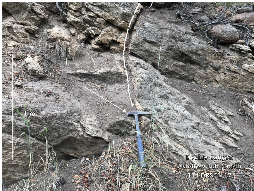
Figure 6-1. Evidence of faulting in the Devine Canyon Ash-flow Tuff (Tmdt) exposed along Forest Road 507 in the northeast corner of the study area disrupted by a small-offset (< 20 cm [8 in]), down-on-the-south normal fault (dashed line) (43.742654, -118.898515 WGS84 geographic coordinates; 4845042mE, 347131mN WGS84 UTM Zone 11 coordinates). Location number: 114 DRSCN 17; Scale bar 1 m (3.3 ft) high; hammer (arrow) 41 cm (16 in) length.
