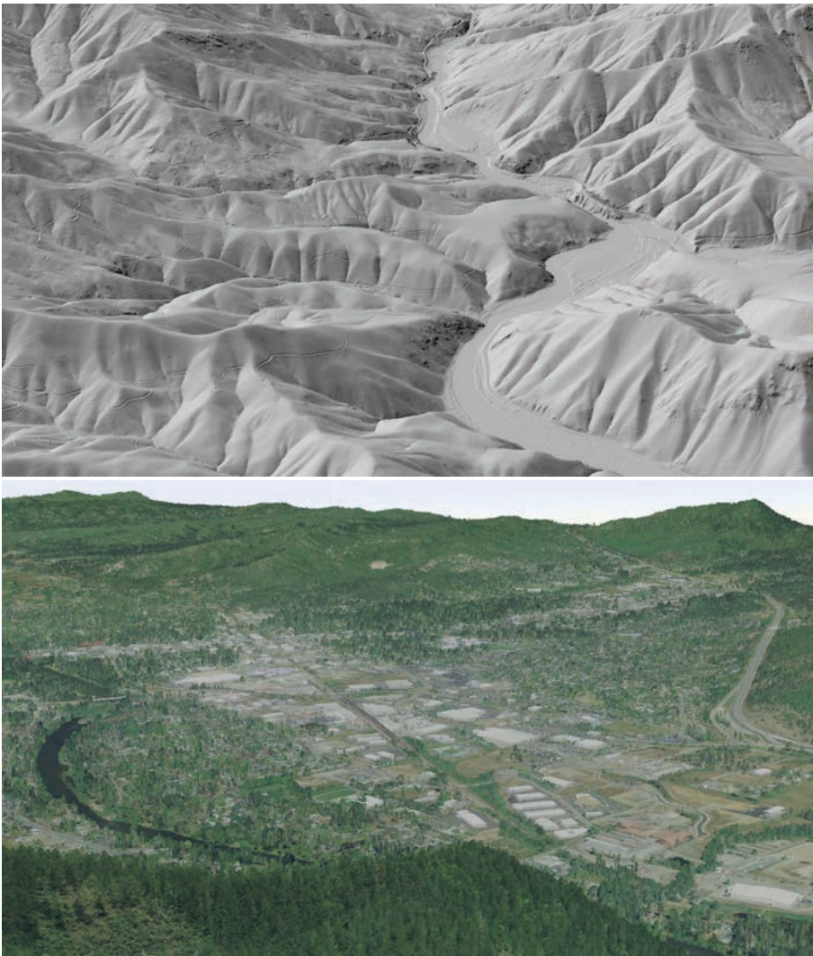
Two ways to use lidar data: (top) Hillshade of lidar-derived 1-m digital elevation model (DEM): Carpenters Island on the Rogue River, Oregon. View to the east. (bottom) Lidar point cloud with RGB extraction from 2009 NAIP imagery: City of Grants Pass, Oregon. View to the north. Images from November 5, 2012, Watershed Sciences, Inc. OLC Rogue River report to DOGAMI.
