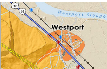
Landslide debris fan (orange) mapped as part of Highway 30 landslide study. Note that the fan crosses infrastructure and a populated area.
