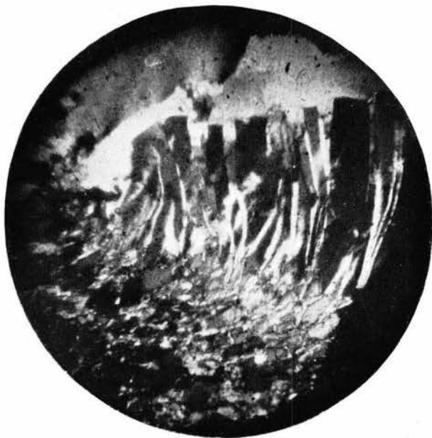
Plate V A. Hornblende with curved cleavages separated by elongated quartz. Photograph of thin section.
