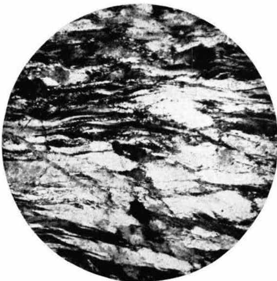
Plate V B. Vein quartz sliced, with some granulation, by shearing. Photograph of thin section.
