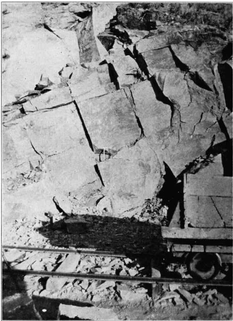
Ideal Quarry, Baker County, showing jointing and size of blocks. Volcanic Tuff.
