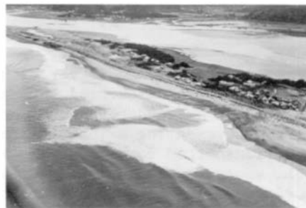
Figure 8: Embayments cut into Siletz Spit by rip currents causing erosion shown in Fig. 7.
