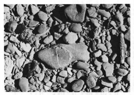
Figure 16. Bedload deposits of gravel along the Rogue River are characterized by high proportions of gravel and low proportions of sand or silt.
