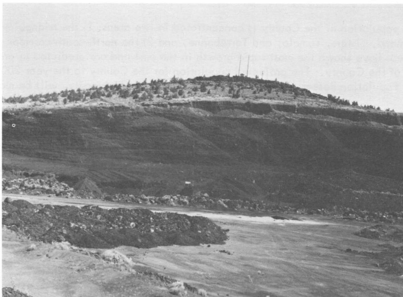
Figure 51. Large cinder pit in sec. 33, T. 14 S., R. 13 E., at south end of Tetherow Butte. Cinders have been dug here intermittently since about 1940, furnishing Redmond and environs with tremendous quantities of aggregate.
