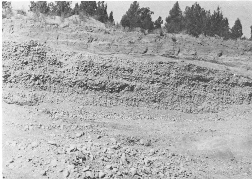
Figure 55. Sand and gravel pit near Johnson Road south of Tumalo, in sec. 6, T. 17 S., R. 12 E. Glaciofluvial fan gravels are overlain by 6 to 12 feet (2 to 4 m) of pumiceous sand and soil and underlain by the pinkish ash-flow tuff unit.
