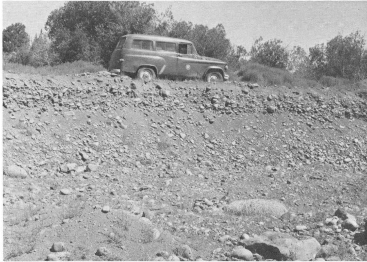
Figure 54. Flood plain and streambank gravels adjacent to Deschutes River north of Tumalo can be mined to depths of 10 or 15 feet (4 or 5 m). Gravels are poorly sorted, containing many large boulders and a high percentage of fine, ashy, and pumiceous material.
