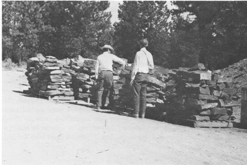
Figure 54. Pallets of black ash-flow tuff rubble stone ready for transport to a Portland market. Stone from this quarry was used for the building shown in Fig. 44.
