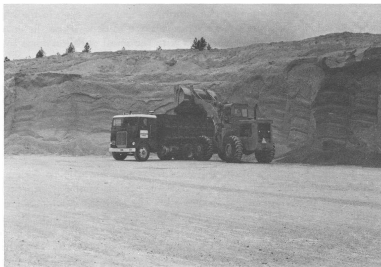
Figure 48. At Central Oregon Pumice Co. pit, after removal of overburden, mining of pumice is accomplished by large front-end loaders and dump trucks. Truck driver generally also operates the loader.
