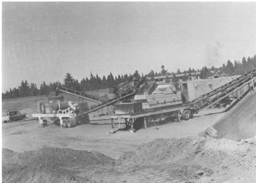
Figure 57. Modern portable crushing, screening, and washing plant of Deschutes Ready Mix Sand & Gravel Co. can produce large quantities of sized material. Pit is in NW \frac{1}{4} sec. 18, T. 17 S., R. 12 E.
