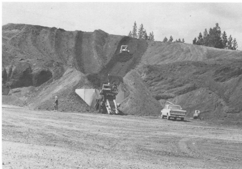
Figure 52. Active cinder pit (1974) has portable screening and loading facility. Near top of Little Pistol Butte. Slopes are smoothed as material is mined.
