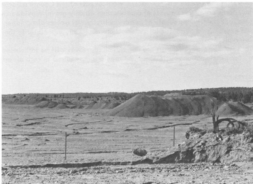
Figure 59. Stockpiles of crushed and screened aggregate from broad shallow pits in an alluvial fan type of sand and gravel deposit near Hampton.
