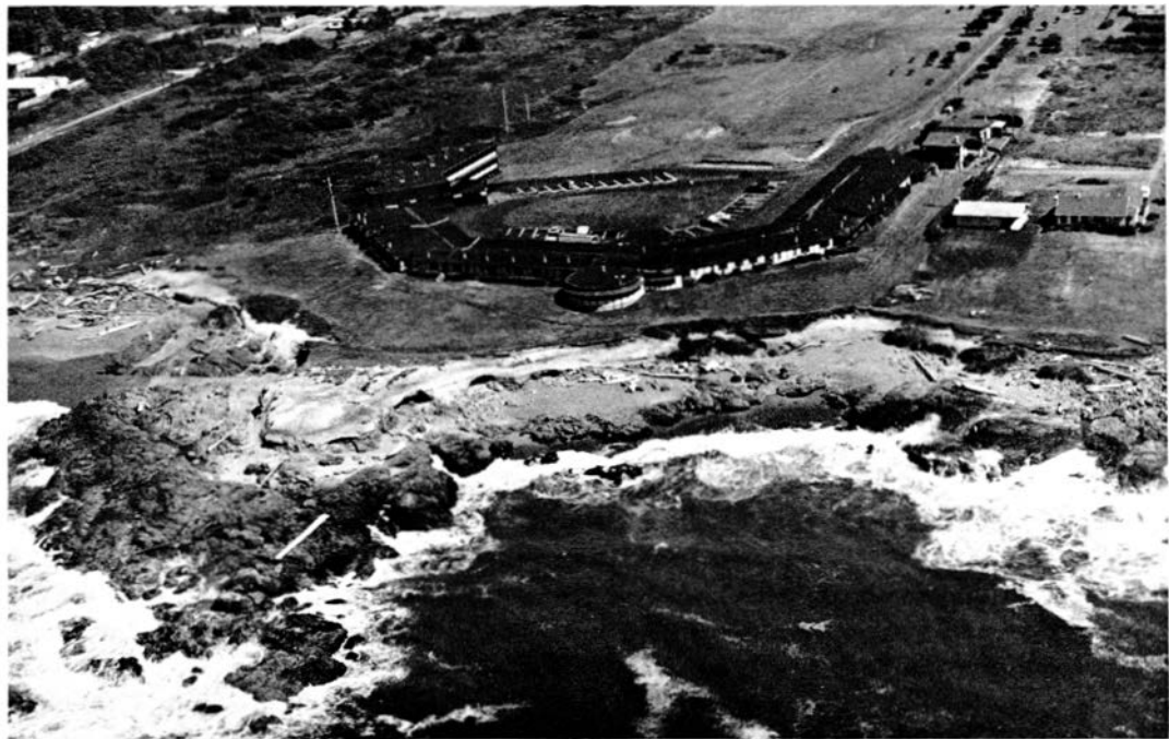
Photo 75. Resistant bedrock underlies marine terrace at this site near Yachats impeding erosion of the thin layer of terrace sands.
