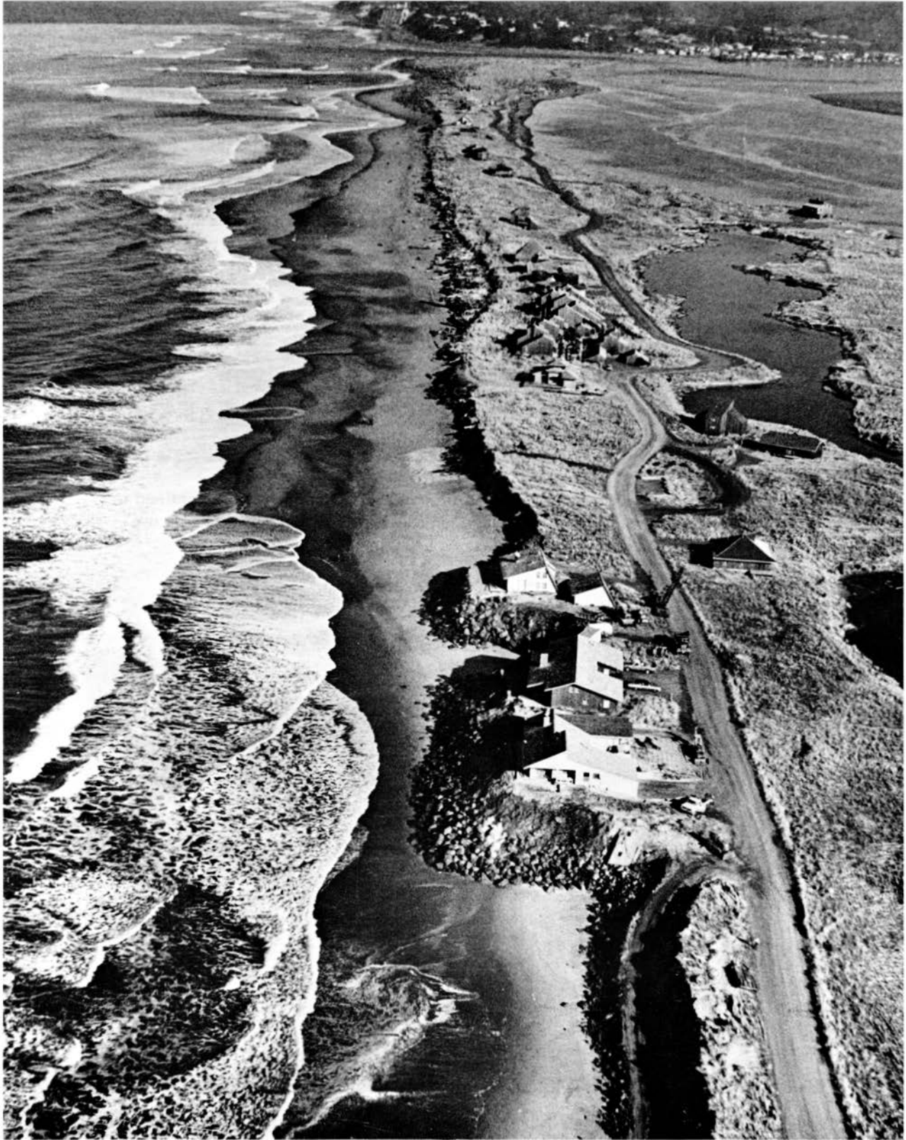
Photo 84. Salishan's development on Siletz spit was severely eroded by winter storms of 1972-73 and required repeated placement of riprap to save houses and property from total destruction. (Photo by Gerry Lewin, Capital Journal )
