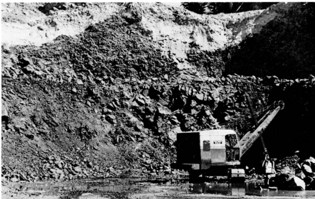
Photo 19. Basalt quarry (No. 33) at Agate Beach. The rock is one of the major sources of crushed aggregate in Lincoln County.
