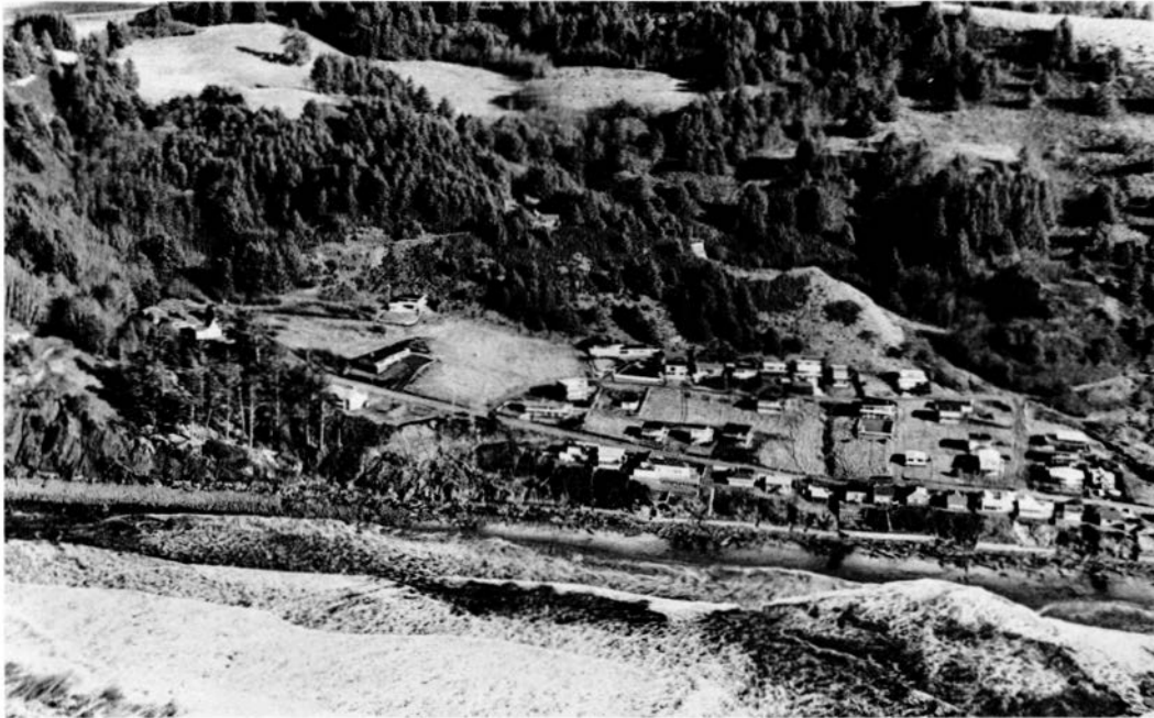
Photo 31. Landslides in sea cliffs at Roods End caused by undermining of weak soils by wave erosion. Remains of house foundation still visible at head of slide in sea cliff near center of photo.
