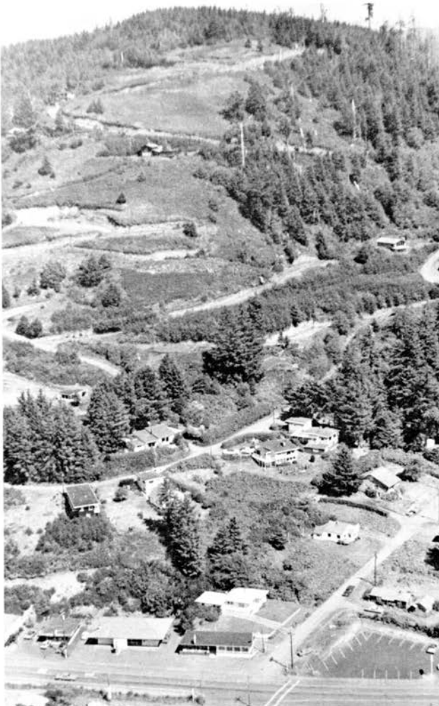
← Photo 86. Homesite development on steep hillside at Yachats must be planned carefully to prevent slope failure in weathered volcanic rock and soils that mantle bedrock.
