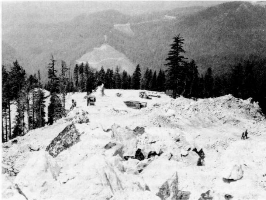
Figure 27. Quarry operations at the Quartz Mountain silica deposit. About 30,000 tons per year are mined, crushed, and screened for use at the Hanna Nickel smelter.
