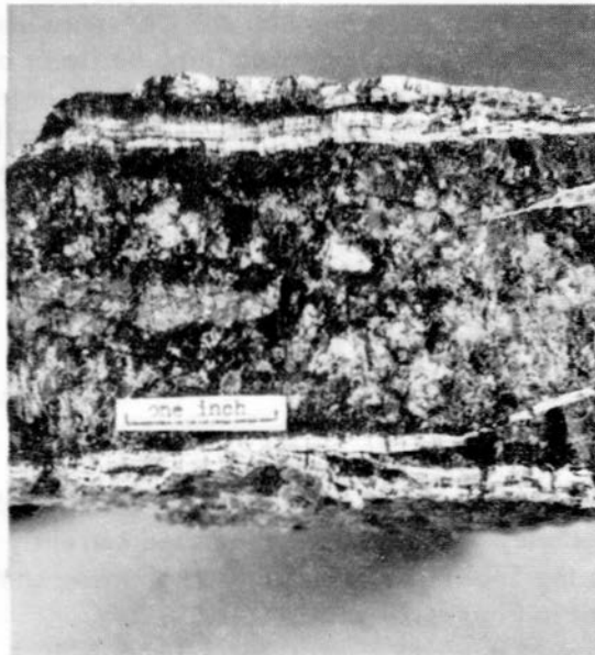
Figure 22. Typical cross fiber chrysotile veinlets in serpentinite; note partings.
