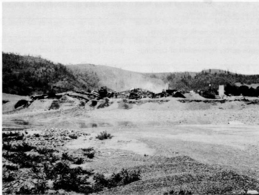
Figure 18. Sand and gravel being screened and crushed from a terrace at Rainbow Hollow on the South Umpqua River. Mineable deposit appears to be about 10 feet thick.
