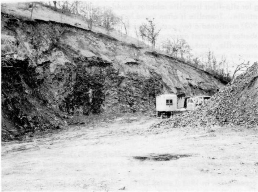
Figure 21. Short and Angel quarry (NW \frac{1}{4} sec. 15, T. 26 S., R. 5 W.) in pillow basalt of the Umpqua Formation is a typical crushed-rock quarry.
