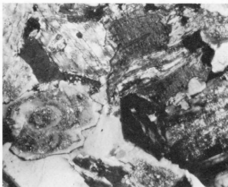
Figure 7. Photomicrograph of the typical Pearse Peak quartz diorite phase, showing characteristic subhedral, zoned and selectively altered plagioclase (left center) with hornblende above and to right, and quartz below. Upper right corner has biotite with prehnite interleafed. (After Kaiser, 1962) (X 45)
