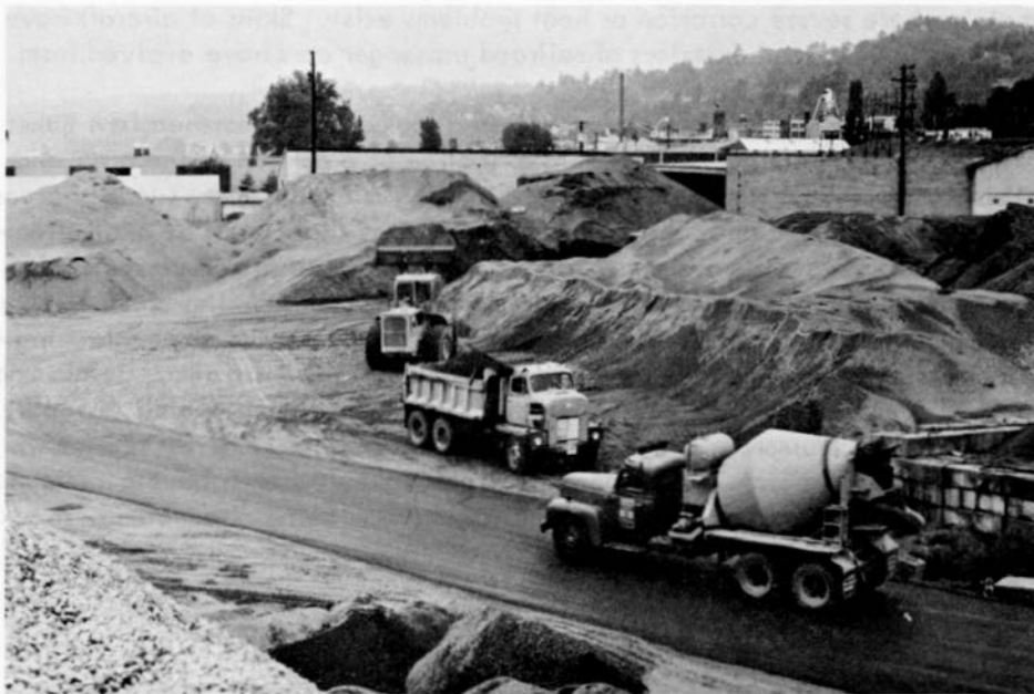
Large aggregate plants supply a variety of products for their customers. Premixed concrete, bituminous mix, and loose aggregate, all tailored for a particular application are shown here in a Portland area sand and gravel plant.
