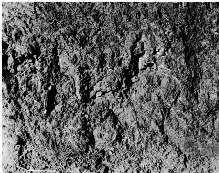
Figure 14. Massive, clayey silt of the Helvetia Formation.
