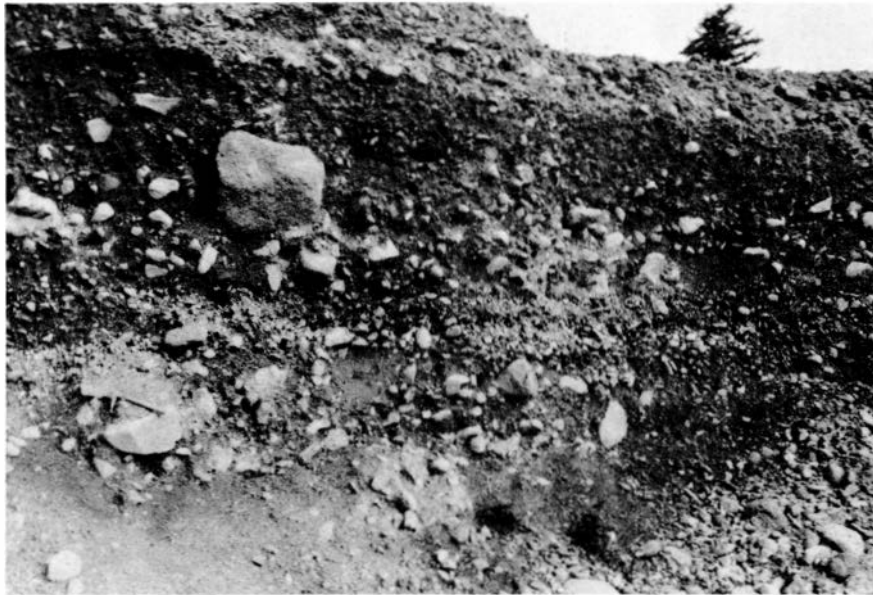
Figure 27. Unsorted silty grovels overlying torrentially bedded grovels at Durham pit.
