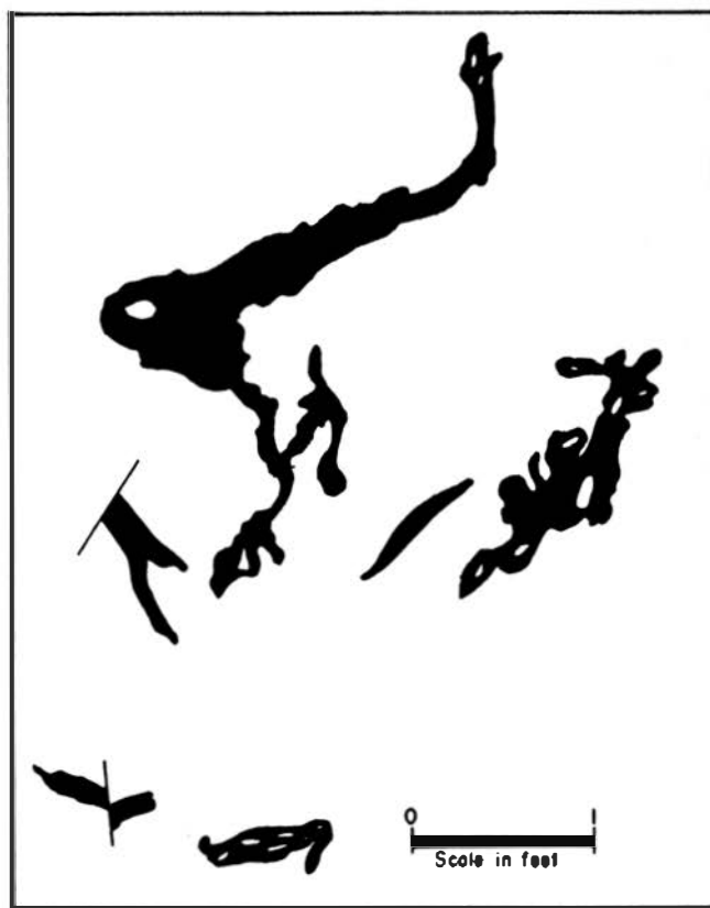
Figure 20. Sketch of massive chromite bodies exposed at Three L claim showing inclosed olivine clots.
