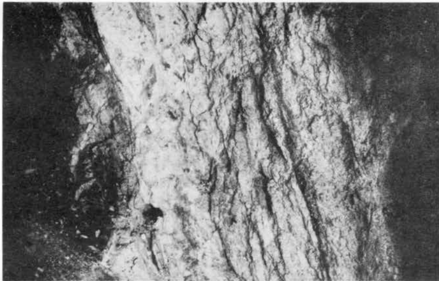
Figure 13 - Constitution vein, level 400, south drift at face (N= 10,270) on September 5, 1957. Footwall not entirely exposed. Across the 18 inches exposed, the vein assayed 0.05 ounce gold and 6 ounces silver per ton.
