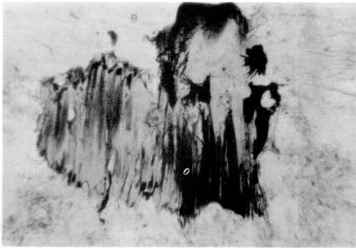
Figure 25-d - Inner green zone. Biotite crystal almost completely replaced by chlorite. Chlorite is light gray; large dark areas are unaltered biotite; and small opaque crystals around edges are pyrite. The radiating needle-like growths are rutile. Width of field is 2 mm. Plain light.
