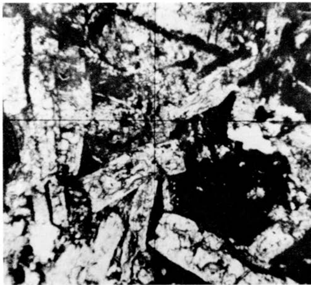
Plate 11 - Photomicrograph of porous granular variety of gibbsite nodule from the Salem Hills. The original texture of parent basalt has been preserved, the plagioclase being replaced by gibbsite. Plain light. Approx. x 55.
