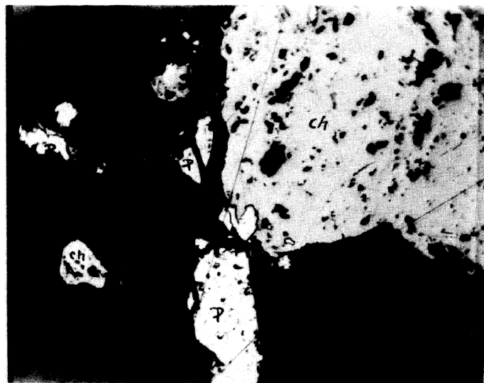
Fig.3. Photomicrograph of ore from the Snow Creek mine. Remnants of pyrrhotite (P) in chalcopyrite (Ch) and with mantles of sphalerite (S). Galena (G) penetrates sphalerite. x 100.
