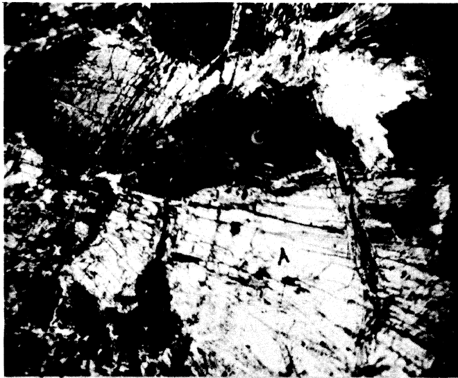
Fig.1. Photomicrograph of amphibolitized dunite. Fibrous masses of actinolite (A) replacing olivine (O). Magnetite (M) is formed in the amphibolitization process. Crossed nicols x 20.
