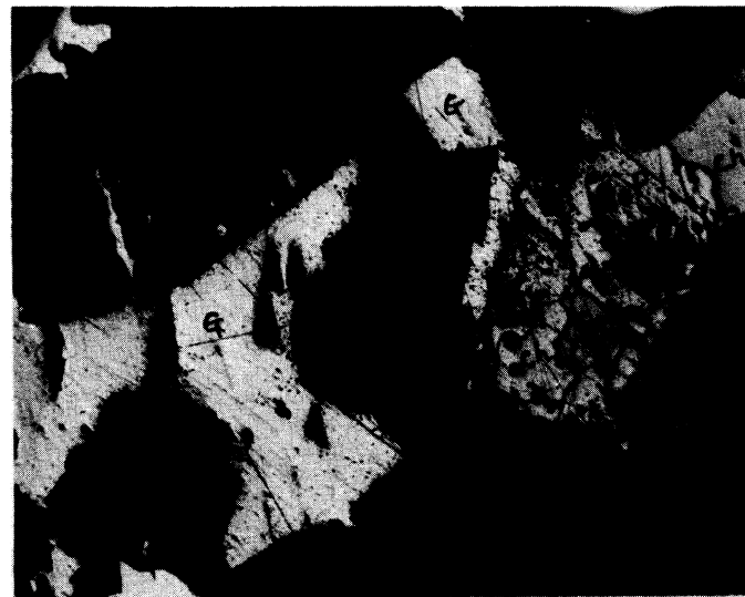
Fig.4. Photomicrograph of ore from Snow Creek mine. Chalcopyrite (Ch) irregularly penetrates pyrrhotite (P). Covellite (Co) is a supergene replacement of chalcopyrite. Galena (G) fills fractures in the gangue and mantles pyrrhotite. x 100.
