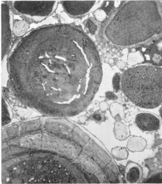
Fig. 1. Photomicrograph of oolitic ferruginous bauxite from Washington County showing differences in the makeup of certain oolites. The matrix is largely gibbsitic material. The white streaks within the oolite to the left of center are gibbsite. Reflected and plain light. Approx. X 15.
