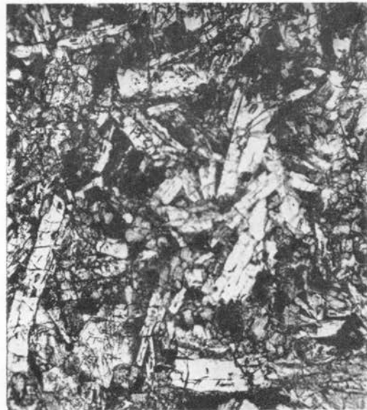
Fig. 4. Photomicrograph of Miocene basalt from Jackson Falls quarry, Washington County. The basalt is made up of labradorite laths, augite, magnetite and glass, and has an intersertal texture similar to those shown in Figures 2 and 3. Plain light. Approx. X 45.
