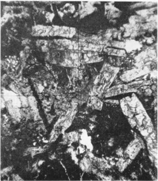
Fig. 3. Photomicrograph of gibbsite nodule from Locality 81, Salem Hills, Marion County. Much of the original texture of the parent basaltic rock has been preserved. The original plagioclase laths have been replaced by gibbsite. Plain light. Approx. X 45.
