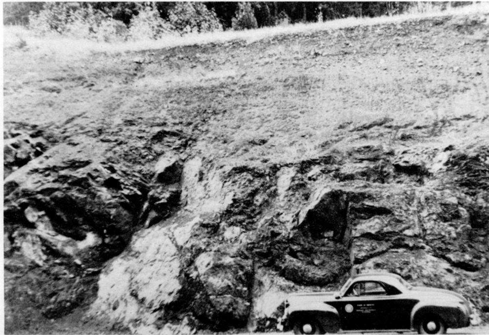
Fig. 1. Road cut on Mt. Sexton, 10 miles north of Grants Pass, Oregon. The photograph shows the formation of soil and the residual mantle rock from fresh rock. Fresh to little altered rock is shown from the bottom of the photograph to a short distance above the top of the car. Considerable alteration of rock is shown about the middle of the photograph and the degree of alteration increases upward. Alteration to soil is essentially complete in the top part of the road cut.
