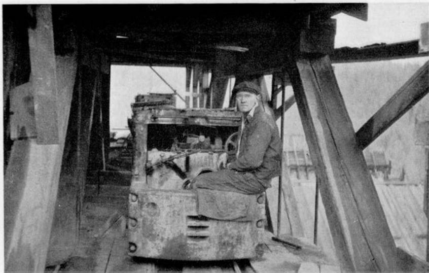
Photo No. 30—Black Butte Mine. Gasoline locomotive bringing a train of ore to the plant from the Dennis Creek Tunnel.
