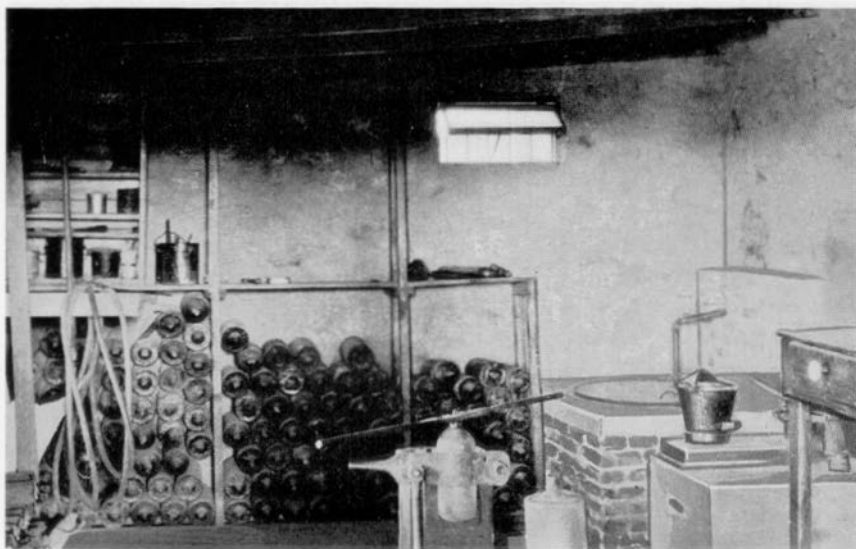
Photo No. 5—A typical "Bottling Room" showing empty flasks in back, full ones at the side and pot, scales, weighing bucket and a flask in the clamp with wrench in place to tighten the stopper.
